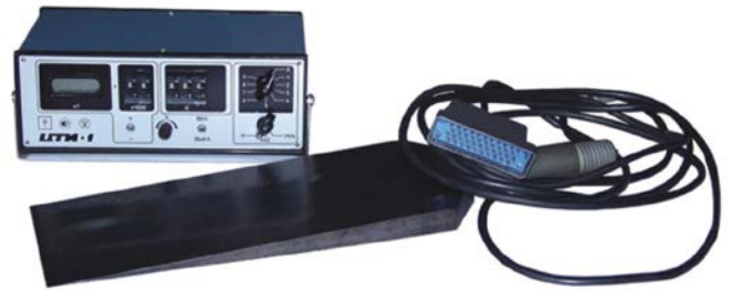
Fig. 4. Wedged dilatometer WD-100, consisting of V-shaped indenter (400 mm high, 100 mm wide, reaming edge expansion angle 4^\circ ), electric cable and digital recorder CTI-1.
